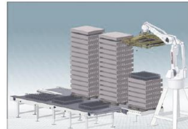
Glass bottle palletizing - full layer handling *
