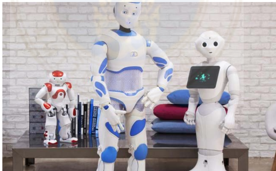
Figure 2.6 Softbank Robotics' robot, from left to right, Nao, Romeo, and Pepper
