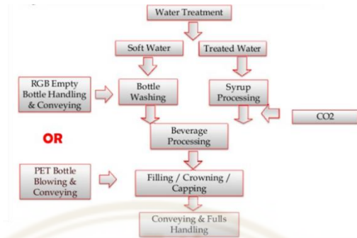
Figure 2.5: Soft drink bottling process (Franson, N.D.)
