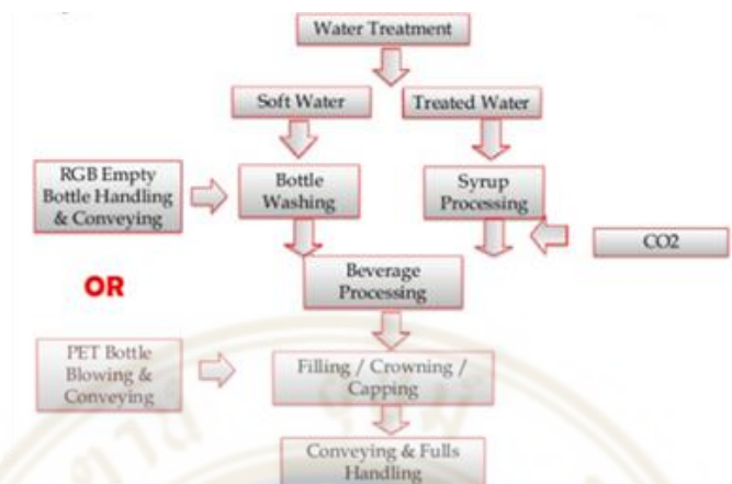
Figure 2.5 Soft drink bottling process
